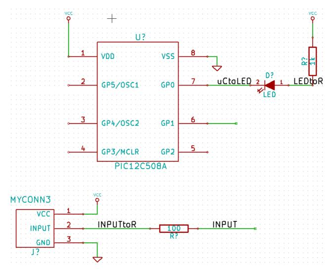
93. The program checks for wiring errors. Any wires that are not connected may generate a warning. To avoid these warnings you can instruct the program that the unconnected wires are deliberate.
