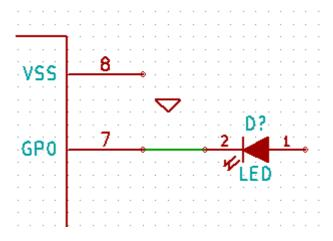
83. Repeat this process to wire up the other components as below. To terminate a wire that isn't connected to anything, double-click the left mouse button. When wiring up the VCC and GND symbols, the wire should touch the bottom of the VCC symbol and in the middle top of the GND symbol.
